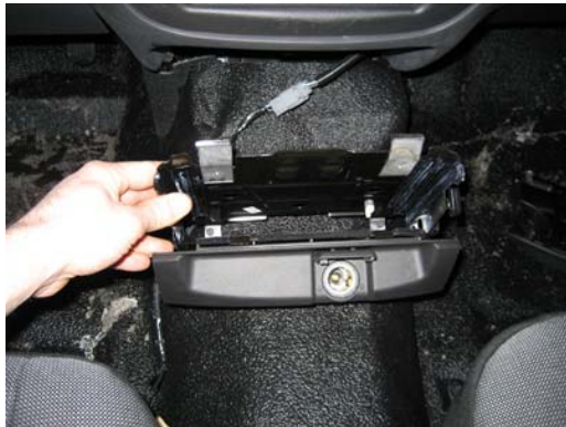
Remove wire plug going to Ashtray/Power point frame assembly
